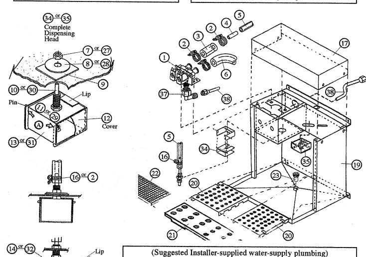
38 QFNCR3 Tube Fitting (Qest)
