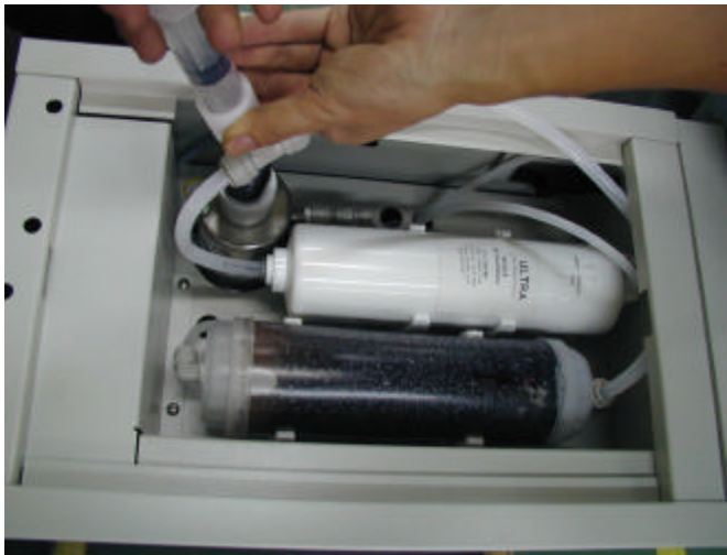
Figure. Sanitization procedure for UF filter
