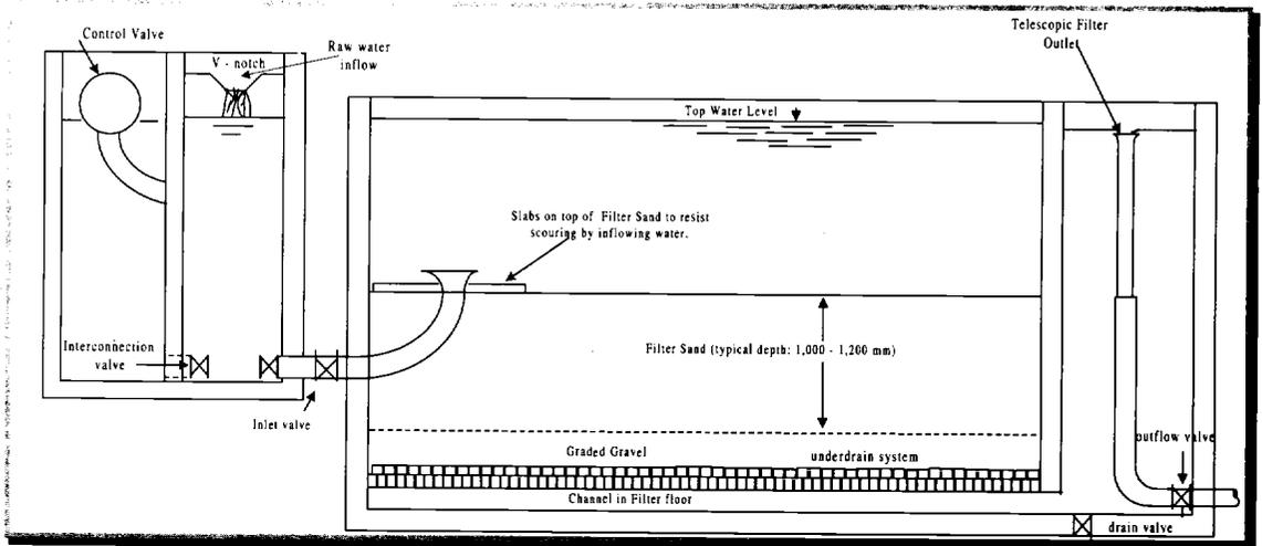
FIGURE 3: SLOW SAND FILTER AND PREFILTRATION CONTROL CHAMBER
