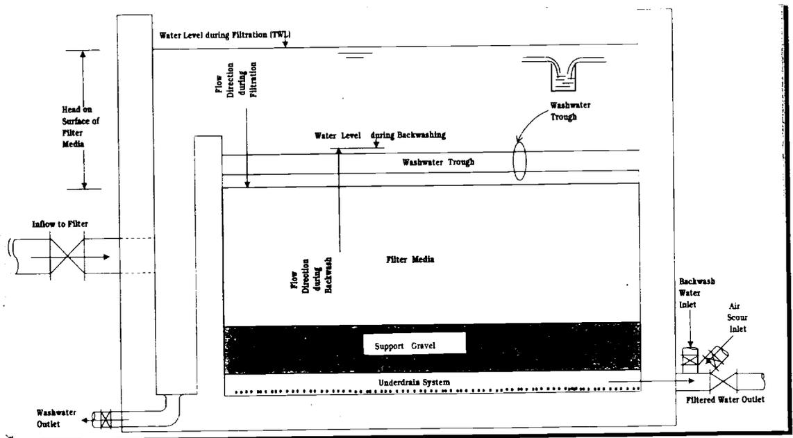
FIGURE 6: RAPID GRAVITY FILTER
