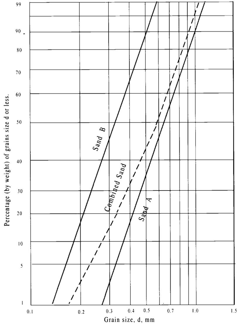
**FIGURE 2: COMBINATION OF TWO TYPES OF STOCK SAND**
