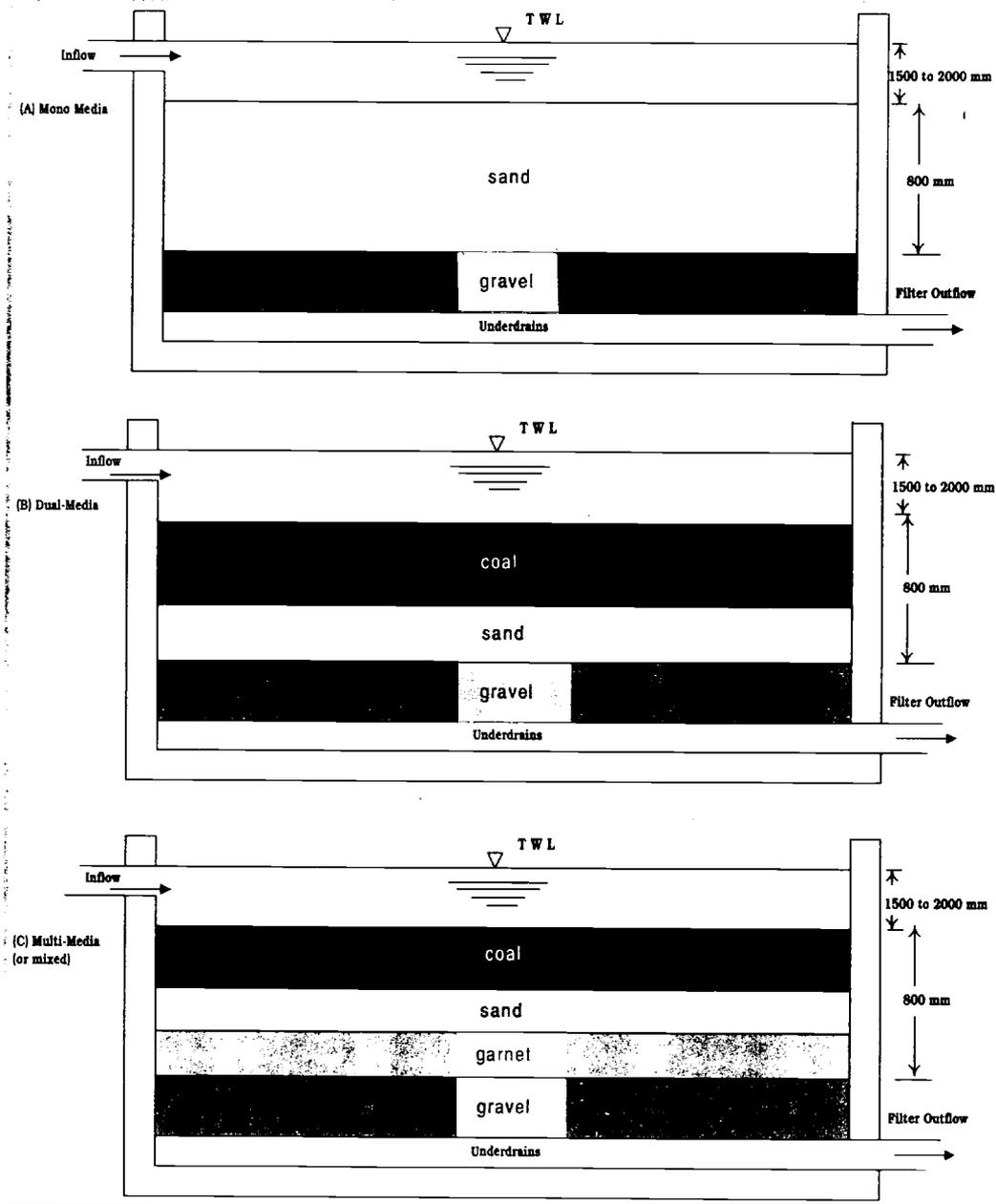
FIGURE 7: GRAVITY FILTER MEDIA CONFIGURATIONS
