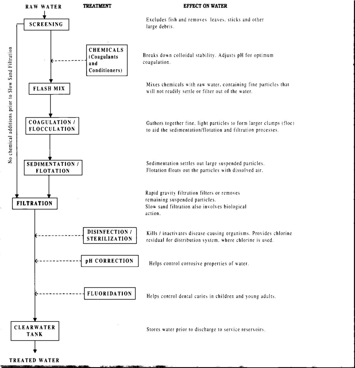
FIGURE 1: TYPICAL WATER TREATMENT PROCESSES
