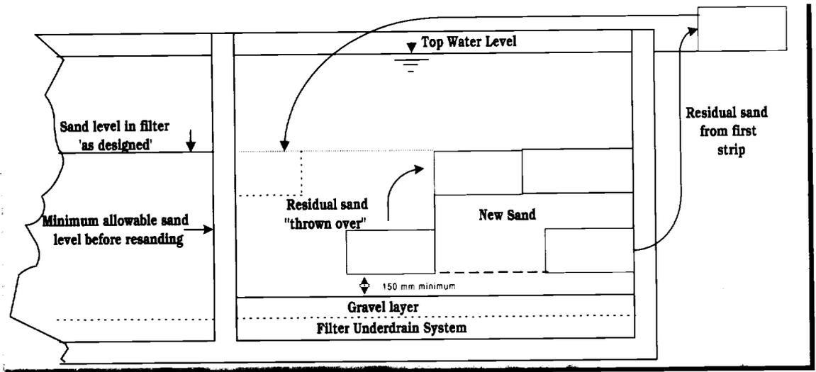
FIGURE 4: REASANDING A SLOW SAND FILTER USING THE TRENCHING METHOD
