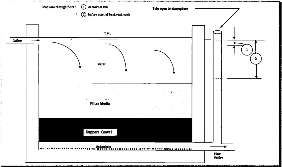
FIGURE 9: MEASUREMENT OF HEADLOSS
