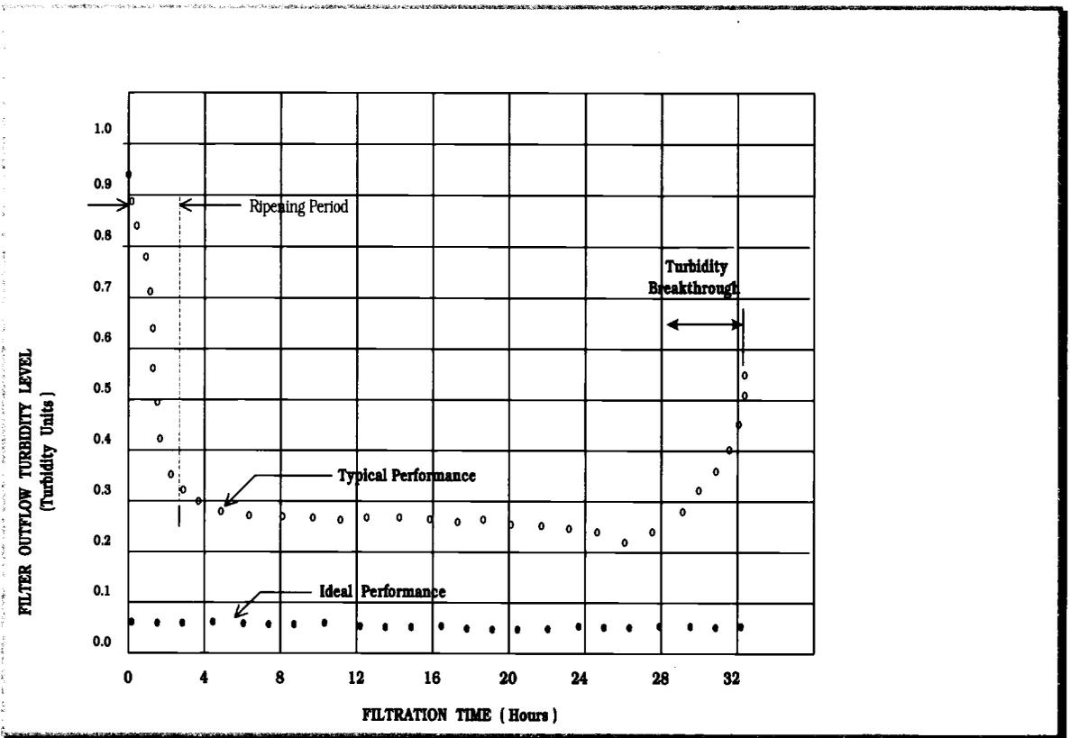
FIGURE 10: TYPICAL OUTFLOW TURBIDITY DATA
