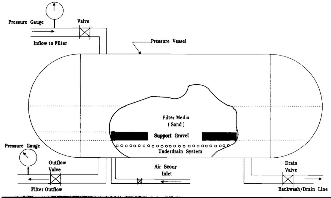
FIGURE 8: PRESSURE FILTER
