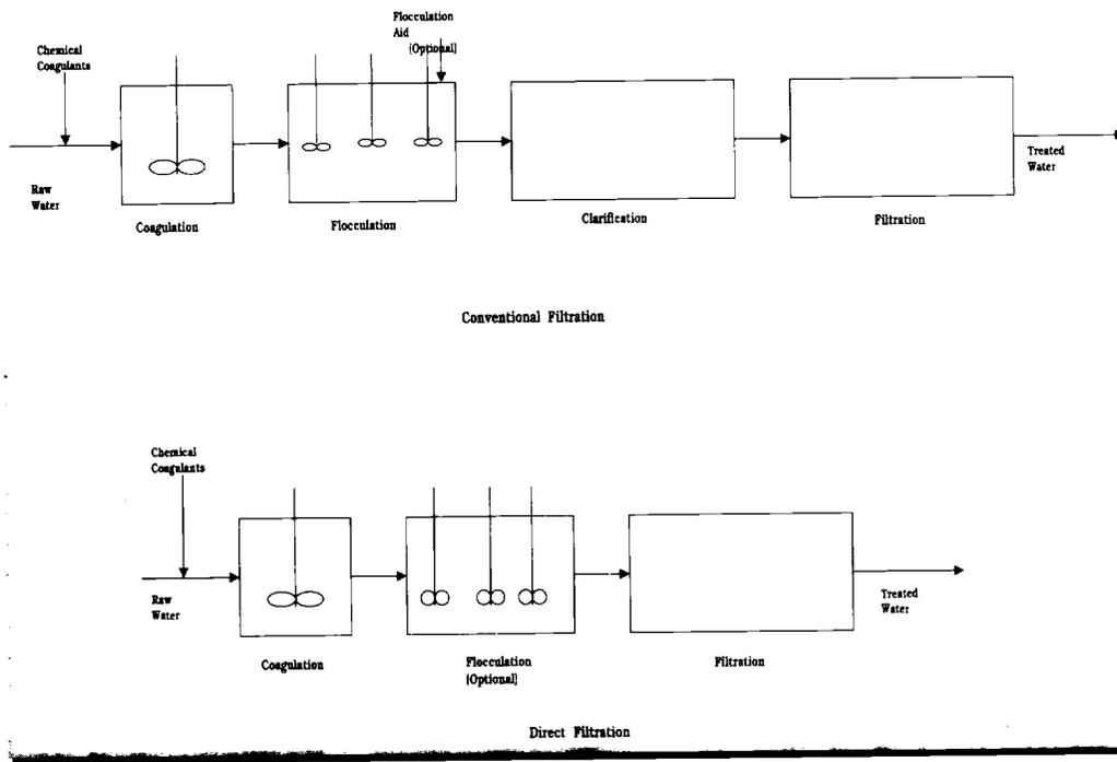
FIGURE 5: CONVENTIONAL AND DIRECT FILTRATION
