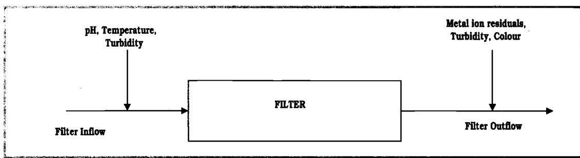
FIGURE 11: FILTRATION PROCESS MONITORING - PARAMETERS AND LOCATIONS
