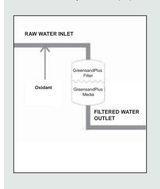
Catalytic Oxidation (CO) operation is recommended in applications where iron removal is the main objective in well waters with or without the presence of manganese. This method involves the feeding of a predetermined amount of chlorine (CI<sub>2</sub>) or other strong oxidant directly to the raw water before the GreensandPlus Filter.
